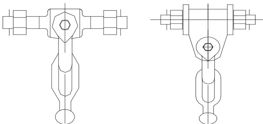
(a) GD Connection method of GD clevis    (b) Connection method of trunnion clevis
