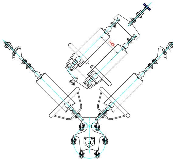
Figure 7-5 Schematic Diagram for Heavy Icy Area Double Joints V String
