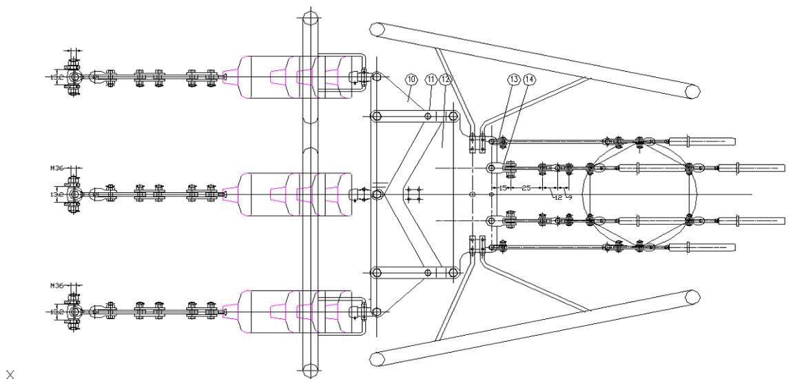
Figure 2-4 Schematic Diagram of Light Ice Conductor 3x400kN Tension String
