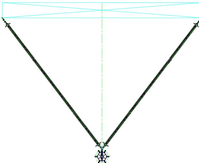
Figure 2-7 Diagram of arrangement of cage rigid jumper
