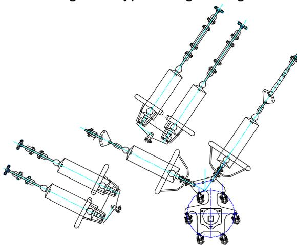
Figure 2-2 Schematic Diagram of L Type String Arrangement in Light Ice Area
