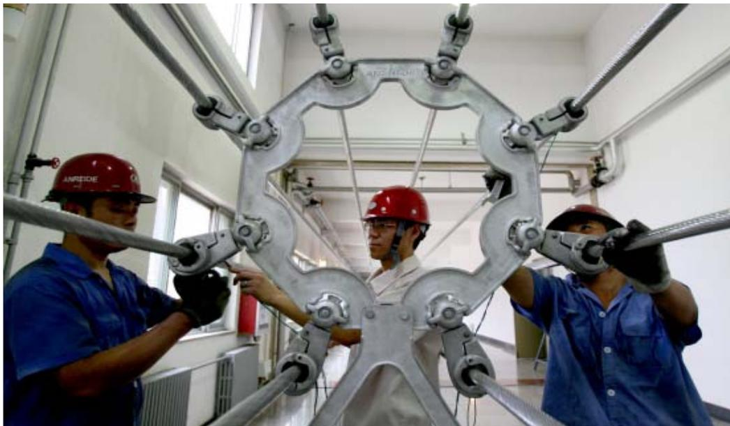
The test of spacer damper
