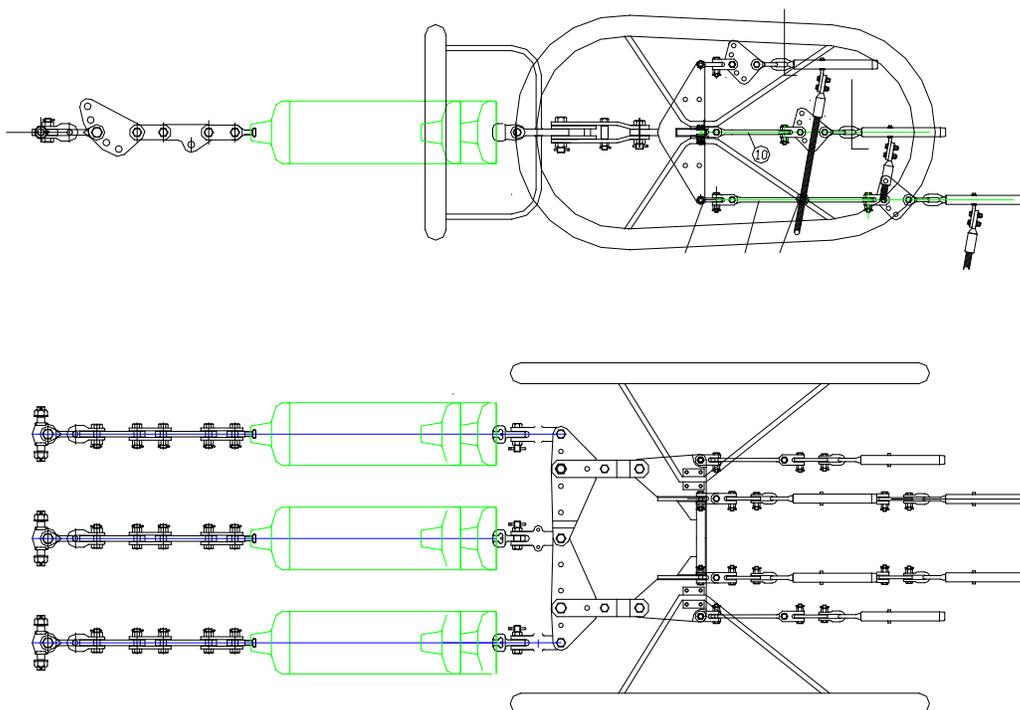
Figure 7-6 Schematic Diagram for 30mm Ice Area Tension String Arrangement
