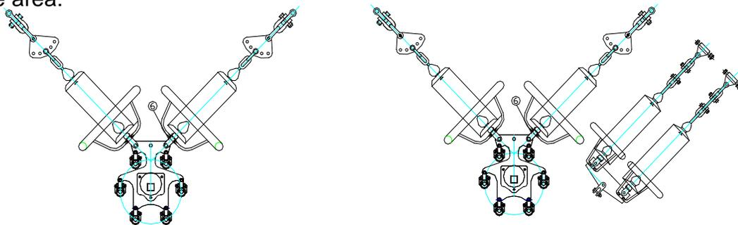
Figure 2-1 Schematic Diagram for Single Joint and Double Joints V String in Light Ice Area
